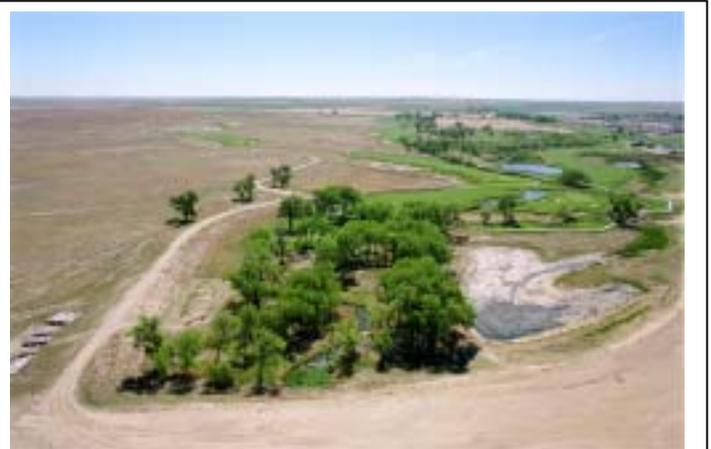
Last year I wrote about the completion of the Green Valley Ranch Golf Course detention facility. Here is an aerial view showing the road embankment that creates the detention, the creek, a water quality pond for local runoff and portions of the 16<sup>th</sup> and 17<sup>th</sup> holes.
