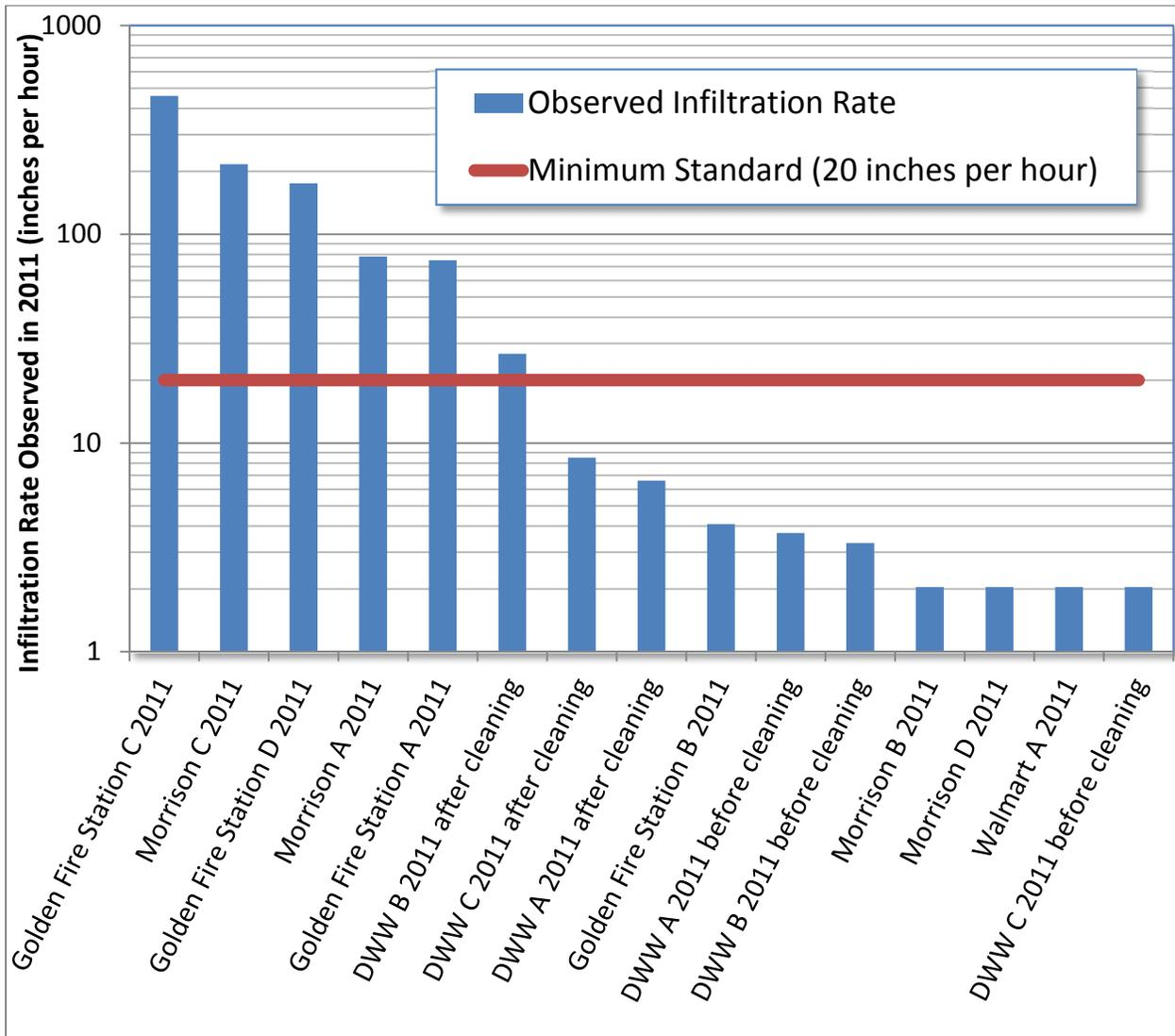
*Infiltration observations at four sites in the UDFCD region. These infiltration rates were observed by UDFCD staff in 2011 using ASTM method C-1701. The Walmart pavement was placed in 2006, the others in 2008.*
