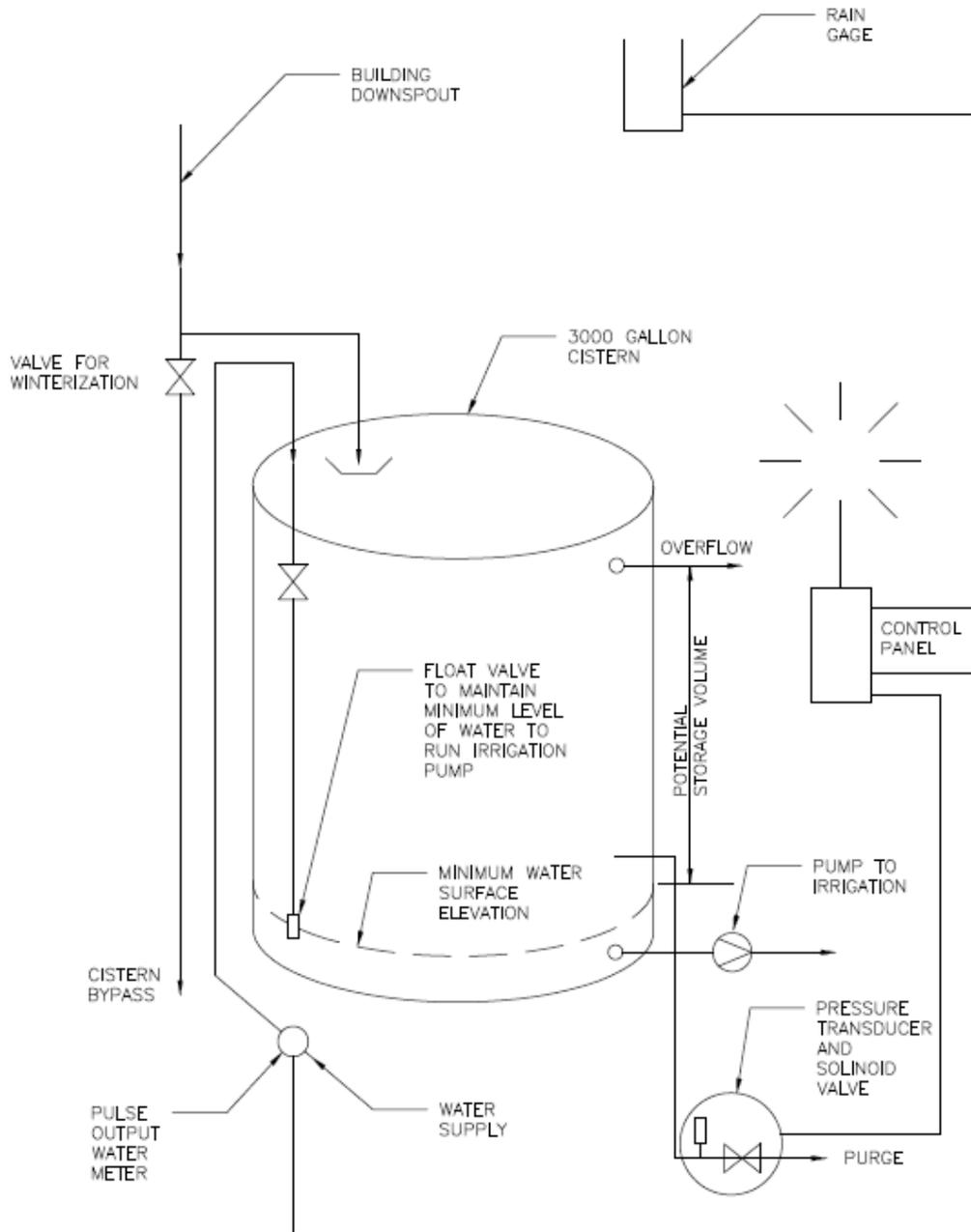
**Figure 1. DGS rainwater harvesting schematic.**
